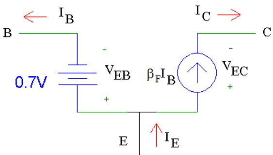
$$V_{BE} = 0.7V \quad V_{CE} > 50mV$$
