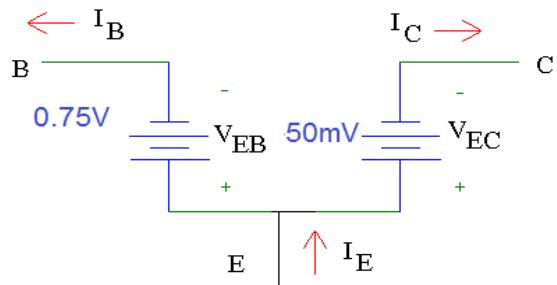
$$V_{BE} = 0.75V \quad V_{CE} = 50mV$$
